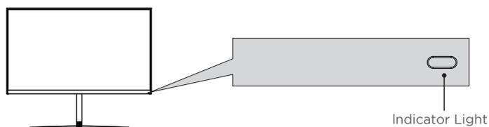
Solid blue light indicates power is on and the monitor is operating normally. Flashing blue light indicates no video source, no horizontal or vertical signal has been detected. Please ensure your computer is on and all video cables are fully inserted and/or connected.
