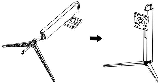
4. Insert the stem to the slot of back cover, then lock them with 4pcs CM4\*26mm screws.( Screws are in the accessory bag, 1pcs buffer )
