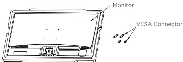
2. Lock the two 26mm VESA connectors in the upper two holes on the rear of the monitor, and the two 10mm connectors in the lower two holes.
