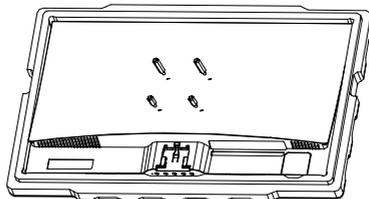
3. Your monitor is now ready to be attached to a wall-mounting bracket. To avoid damage, please do not pinch the screen during bracket installation.
