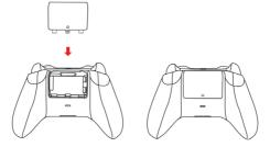
Remove the battery cover of Xbox One<sup>™</sup> controller, then slide the rechargeable battery into the battery bay. 3
